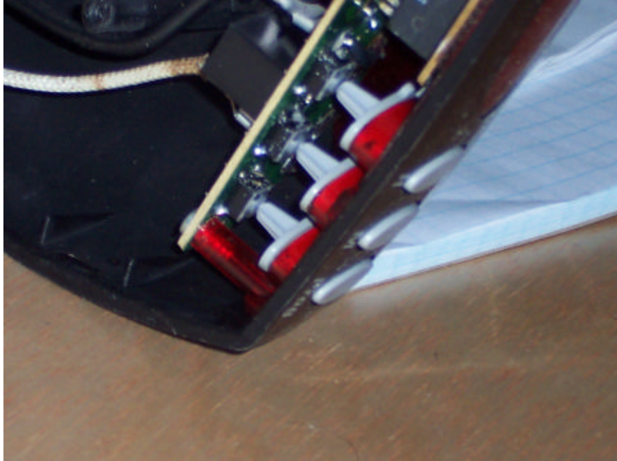
PCB switches in a cheap coffee maker.
